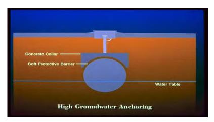
*Illustration of adding a concrete collar at the top of the tank to offset buoyancy*
