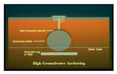
Illustration of hold-down pad installation under the UST to offset buoyancy
