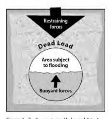
Figure 1. Tanks are typically buried 3 to 4 feet below finished grade to provide adequate slope for piping and protection from traffic loads. Except in areas with high water tables or areas subject to flooding, the weight of the backfill and pavement over the tank is sufficient to offset buoyance and prevent flotation.
